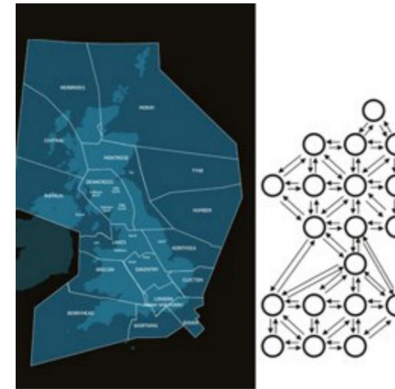
A graph representation of the simplified airspace model used with regions being represented by nodes and borders by vectors.
