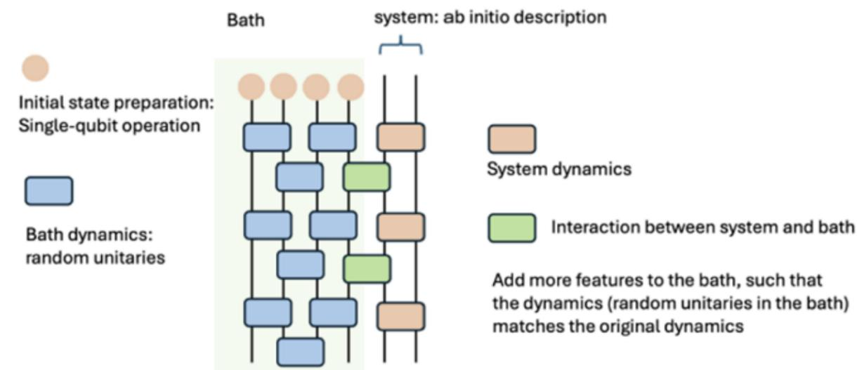
Schematic of the full quantum system circuit. The objective is to obtain an effective description of the quantum dynamics of the distant part of the system. To achieve this, the full, large system is divided into the bath and the system.
