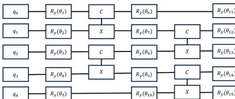
Figure 6. Example of VQE parameterised/quantum circuit with 5 qubits.
