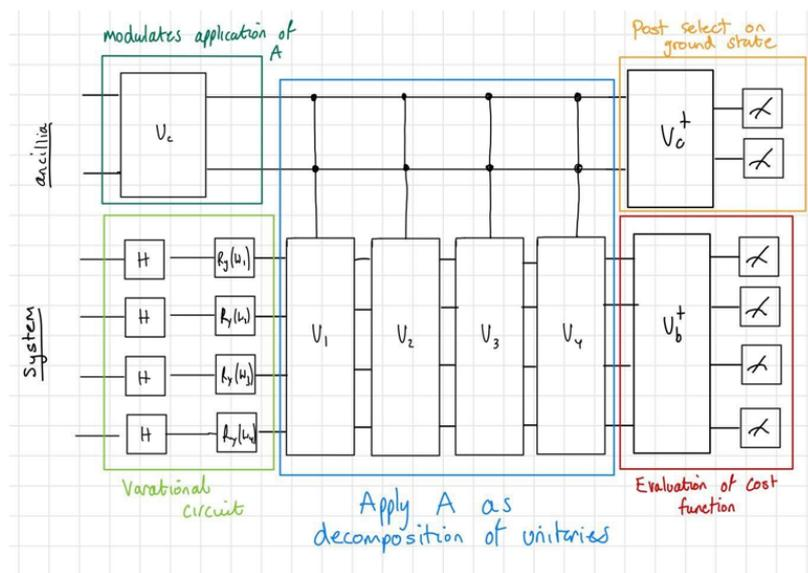
Figure 4. Circuit for the CVQLS with descriptions of the different portions
