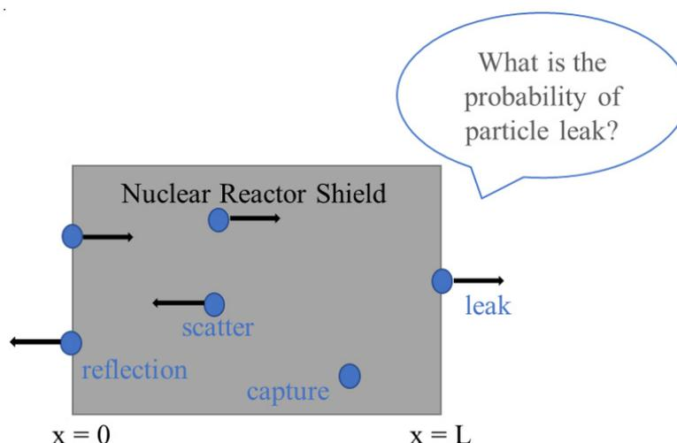
Figure 3. Example of particles travelling through a 1-D shield of length  $L$ .
